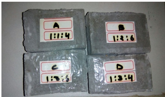
Fig. 1: Specimens of grout in different ratio
